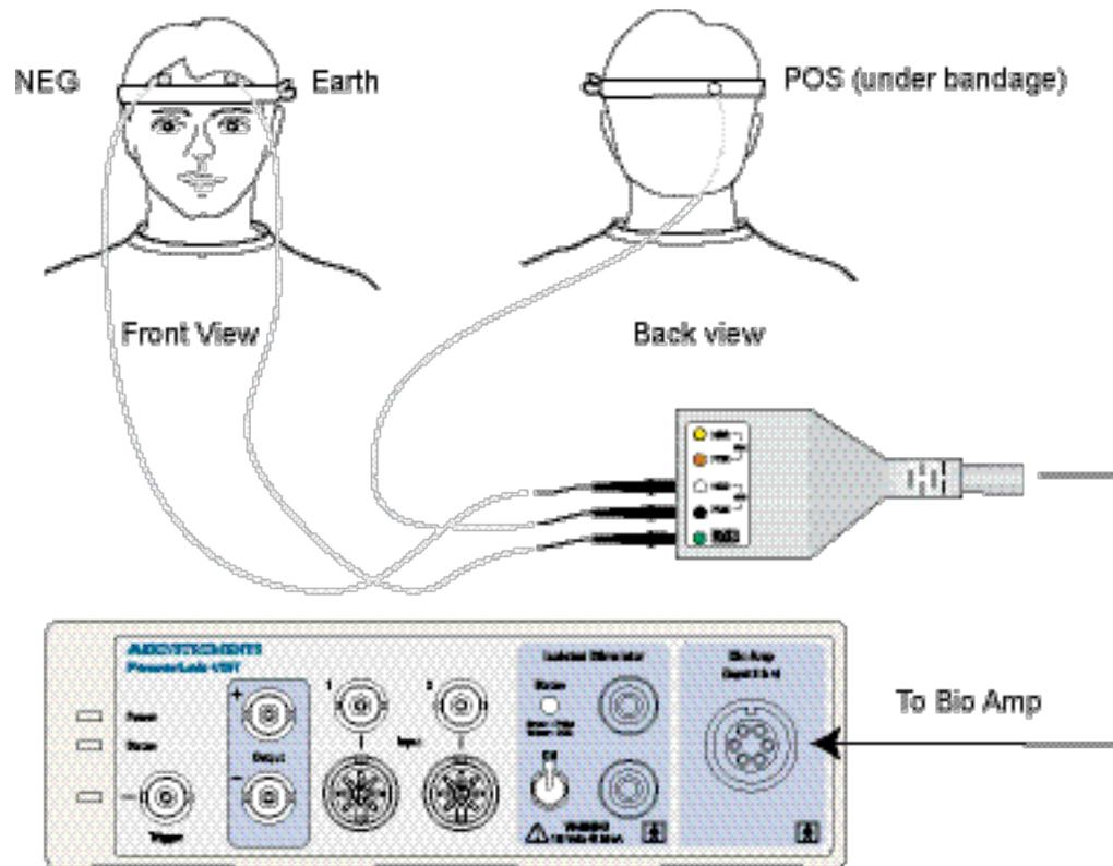
Figure 1. The equipment setup for this experiment, showing the placement of EEG Flat electrodes on the head of the subject.
