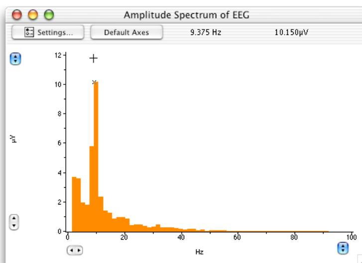
Figure 6. The spectrum of an EEG: the Waveform Cursor is placed over a prominent peak, showing alpha wave activity in the range 8–12 Hz.
