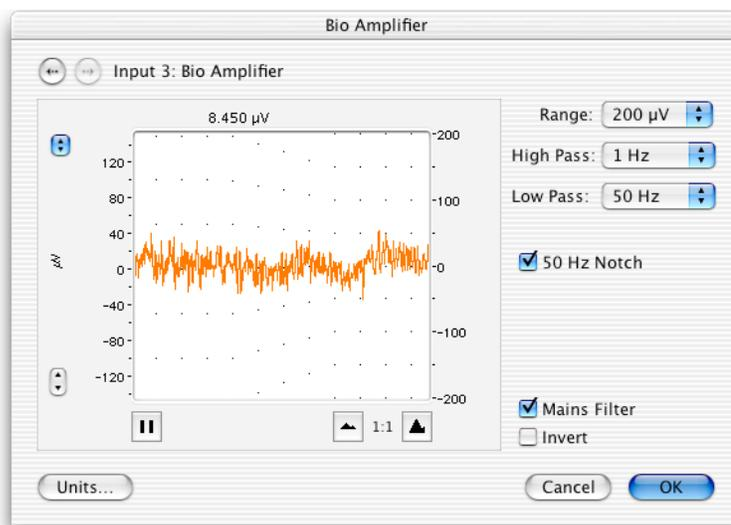
Figure 3. The Bio Amplifier dialog, showing settings for EEG.
