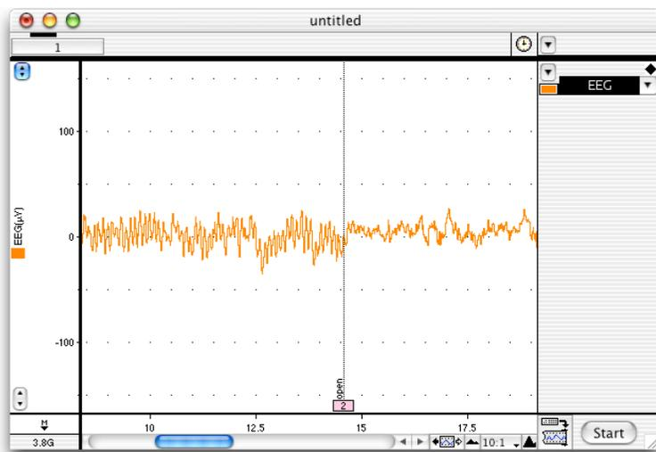
Figure 4. An EEG, viewed with a 10:1 horizontal compression. Alpha waves show as fine oscillations that stop when the eyes are opened (comment 2).
