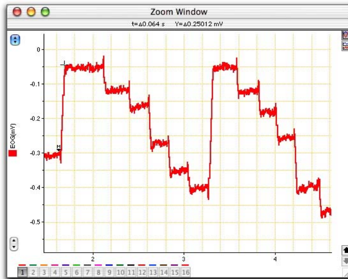
Figure 4. Saccades during reading. Note the position of the Marker and Waveform Cursor.
