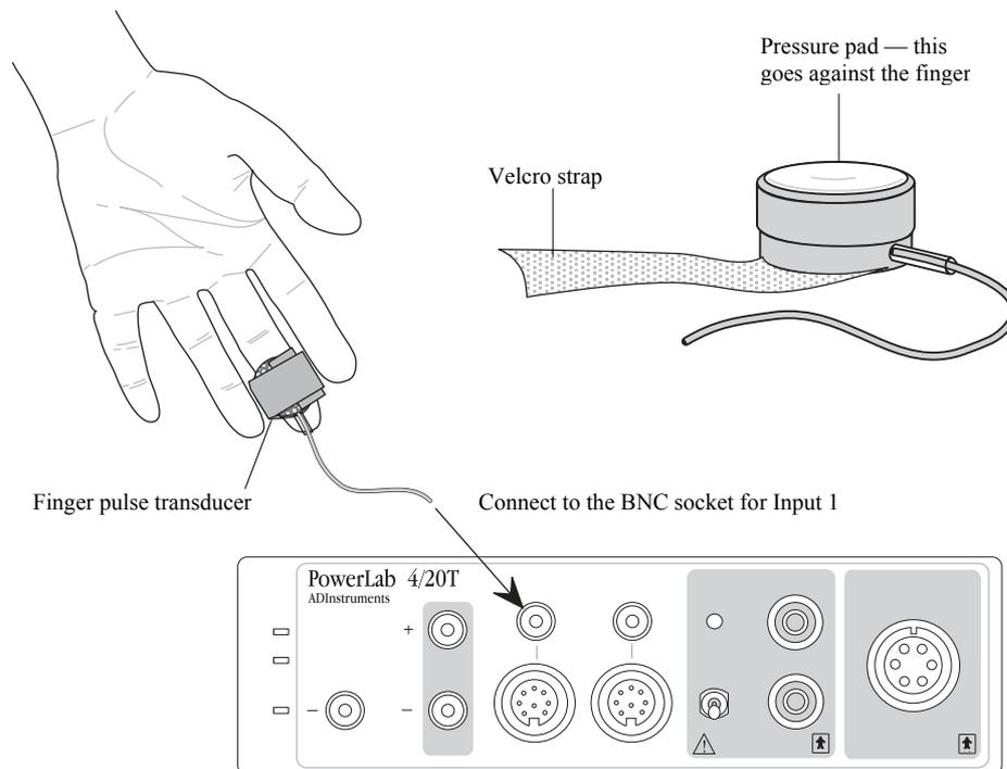
Figure 5. How to connect the finger pulse transducer to the PowerLab and the finger.
