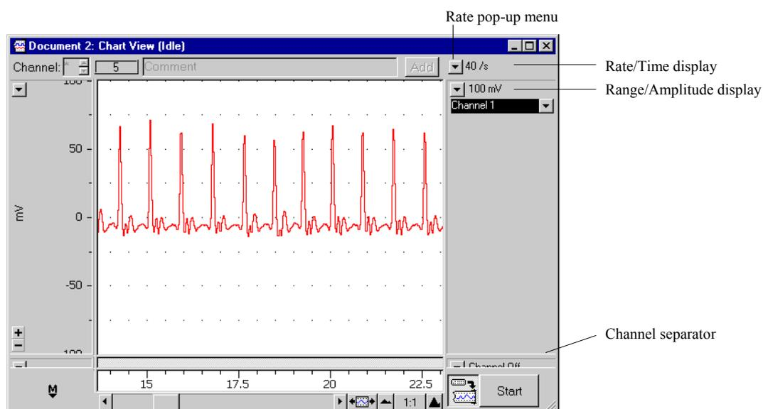
Figure 7. An example of the sort of waveform you should see with the finger pulse transducer.
