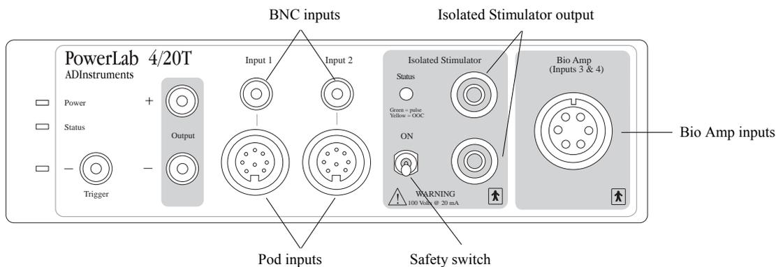
Figure 2. The front panel of the PowerLab 4/20T.
