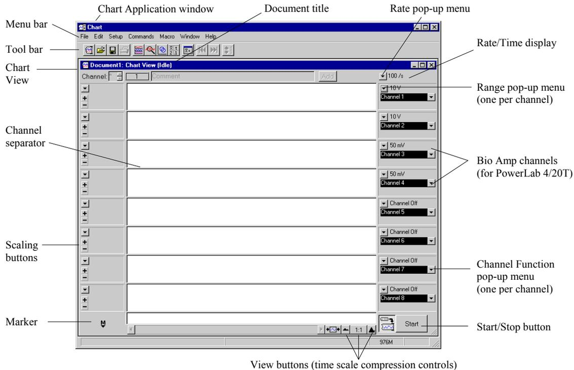
Figure 3. Chart's menu bar, Tool bar and Chart View.
