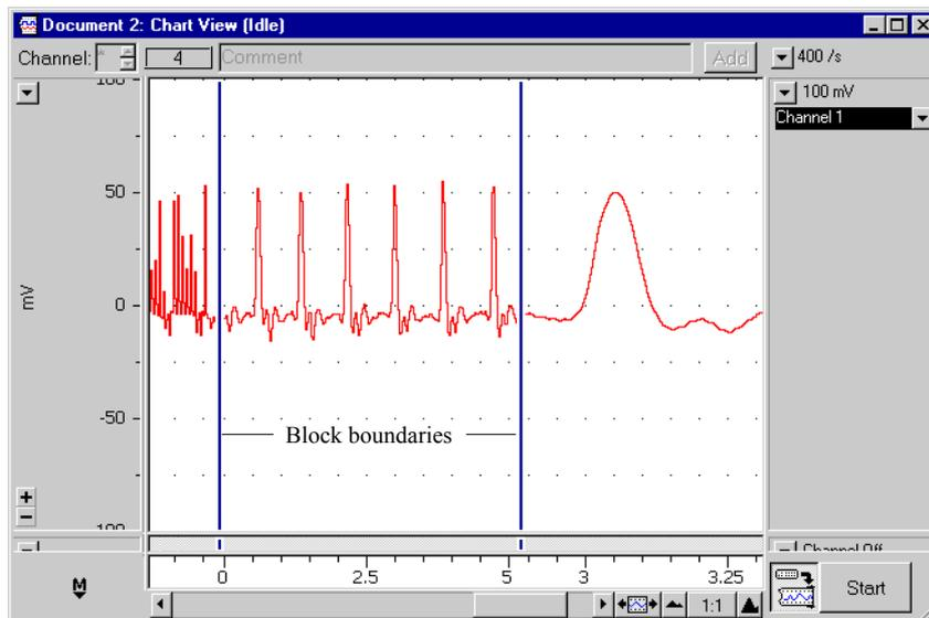
Figure 8. An example of the type of waveforms you could see when changing sampling rates.
