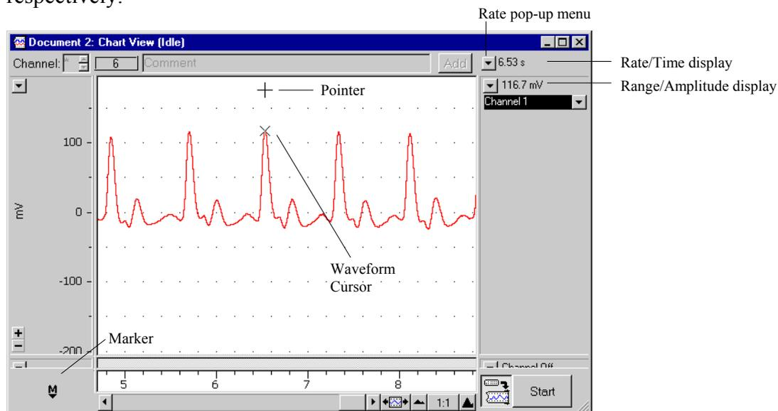
Figure 10. Measuring values with the Waveform Cursor.
