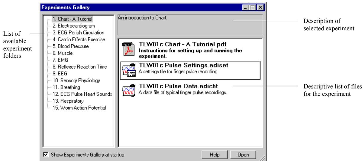
Figure 4. The Experiments Gallery dialog box, with the settings file for this experiment selected.
