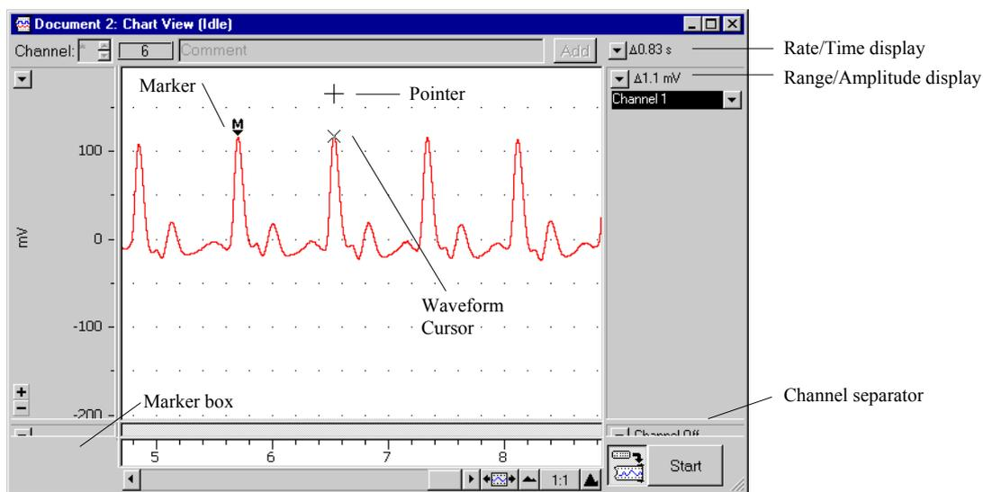
Figure 11. Measuring values with the Waveform Cursor and Marker.
