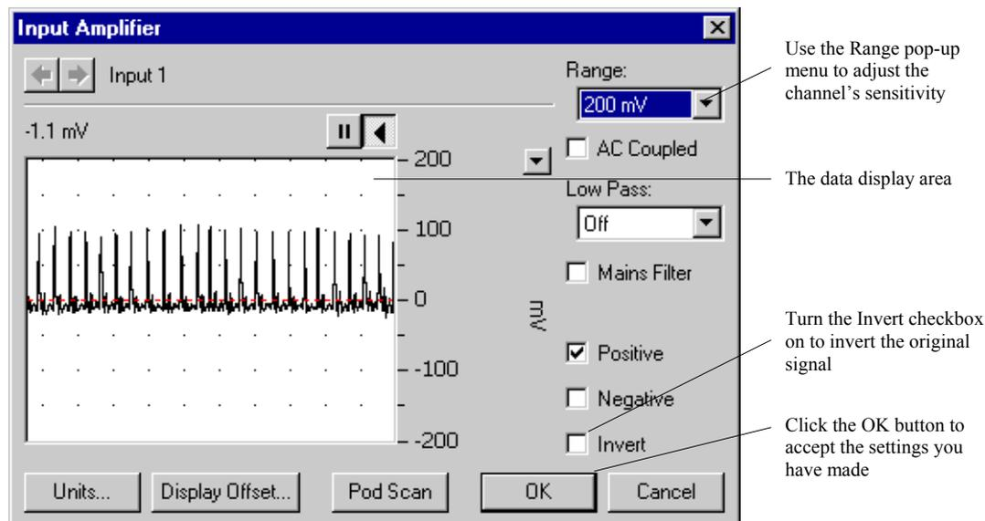
Figure 6. The Input Amplifier dialog box.
